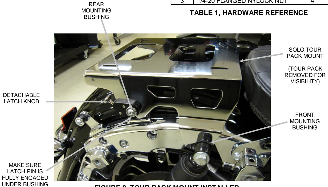
FIGURE 2, TOUR PACK MOUNT INSTALLED
