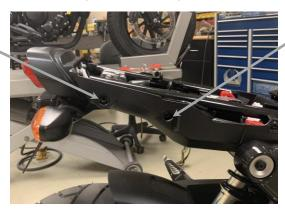
FRONT MOUNTING LOCATION (REMOVE PLASTIC COVERS TO EXPOSE THREADED MOUNTS)
