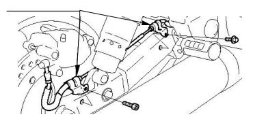
2. Install your new swingarm cover using the supplied M6 button screws making sure the brake hose clamps are positioned as shown.
